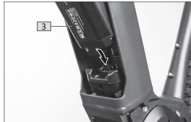
3. Press the battery (3) back into the down tube with both hands.
